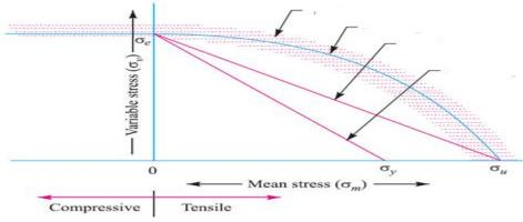
15. Write Soderberg's equation and state its application to different type of loadings.
