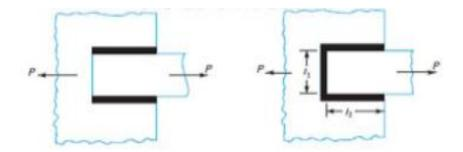
27.A 65 mm diameter solid shaft is to be welded to a flat plate by a fillet weld around the circumference of the shaft. Determine the size of the weld if the torque on the shaft is 3 KN-m. The allowable shear stress in the weld is 70 MPa
